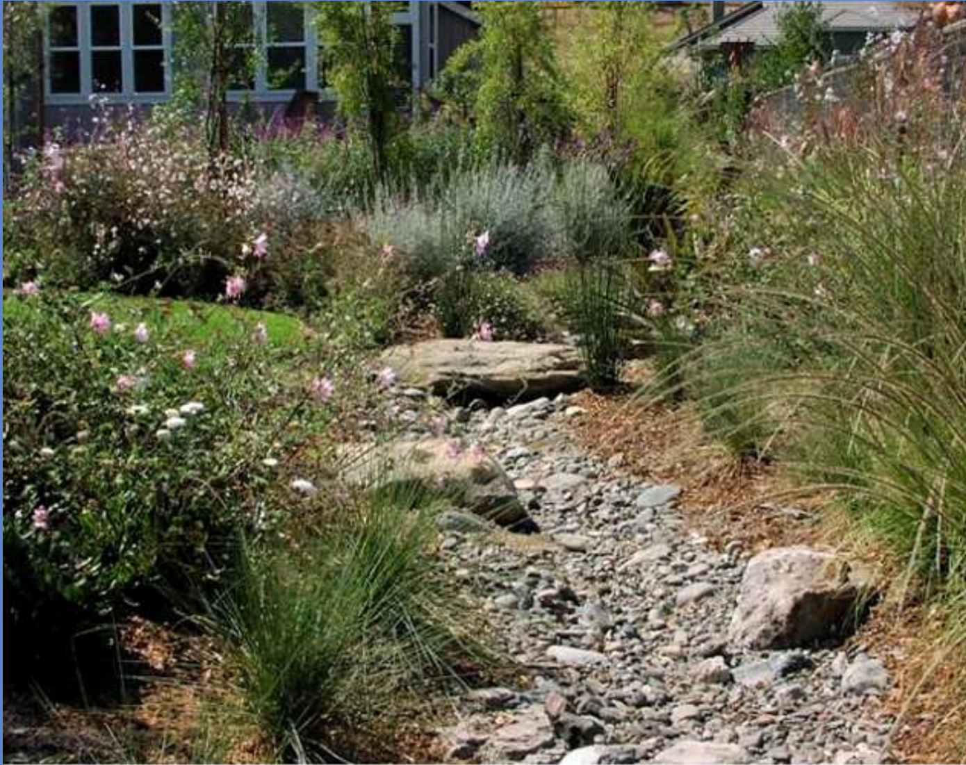
Novato, aesthetic top dressing to drainage system -dry stream bed look.
